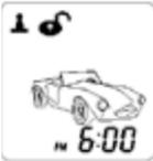
**PATHWAY ILLUMINATION** This feature turns the parking light "ON" for 30 seconds upon a unlock signal and for 10 seconds upon the lock signal.
