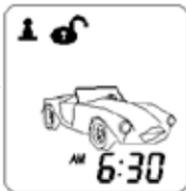
The vehicle will shut down and turn off the parking light to indicate engine stopped.
